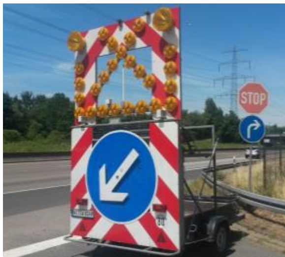
Figure 16: Road Works Safety Trailer, operated by Hessen Mobil, Germany Source: Sandro Berndt, BAST
